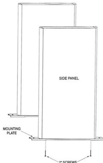
**Caution:** Adjust the width of the unit at the bottom of the panels to 30" (762mm) BEFORE making the holes in the next step.
